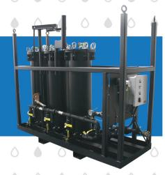
The Model 503 is a turnkey filter system designed for high-flow filtration of large reservoirs up to 7,500 gallons in capacity. The Model 503 utilizes kidney-loop filtration to continuously clean your fluid. With COMO, you can extend fluid and machine life by removing particulate down to 1 µm and water contamination to as low as 20 ppm.
