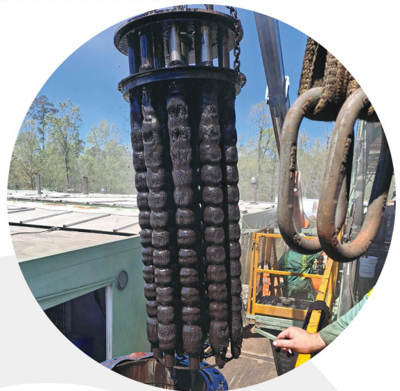
In 6 hours, these magnetic filter elements captured 100 lbs of contamination under 4 microns
