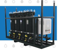
The Model 504 is a turnkey filter system designed for high-flow filtration of large reservoirs up to 10,000 gallons in capacity. The Model 504 utilizes kidney-loop filtration to continuously clean your fluid. With COMO, you can extend fluid and machine life by removing particulate down to 1 µm and water contamination to as low as 20 ppm.
